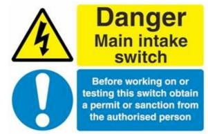
Example of electrical warning sign with mandatory instructions for example for use with multiple supplies, remotely/automatically controlled generating sets, main Intake Switch Sign, switch off electrical equipment before working etc.
