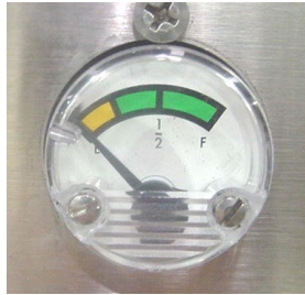
Differential Pressure Gauge (2)
