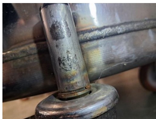
This wheel came off due to a design flaw which caused it to become unstable and injured the person moving it!
