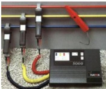
The monitoring equipment is ideal for site surveys and monitoring specific tasks as it causes minimal disruption. It monitors supply and consumption by means of safe non-contact current transformers. These can be placed around conductors without the need to switch off the power and without the need for live electrical contact.
